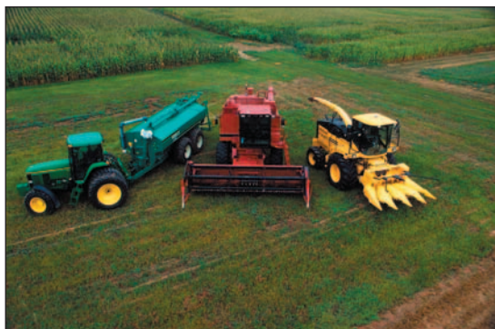
Many farm machines at ARS' Beltsville Agricultural Research Center run on a mixture of diesel fuel and biodiesel, which is made from soybean oil. Photo by Bob Nichols. Courtesy of USDA/ARS.
